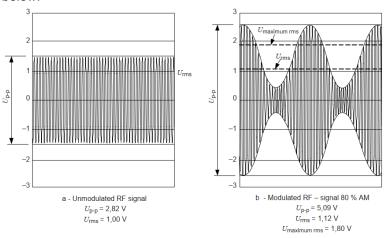
Because the RMS level of the modulated signal must match the test level, the peak amplitude of the modulated signal must be 5.1 dB greater than the RMS amplitude of the test level specified by the standard.
